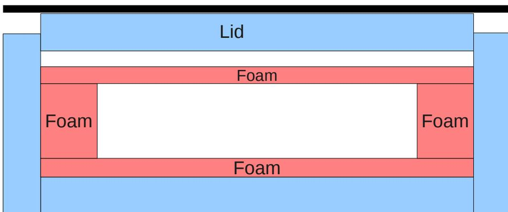
Foam is in three sections, top, middle and bottom
